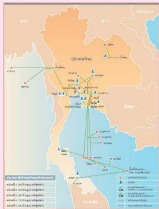
Today (2008) the pipeline network of PTT across the country both onshore and offshore stretches over a distance of 3,100 kilometers. The network is transmitting over 3,500 million cubic feet per day (MMscfd) of natural gas to be used as fuel for the power plants, industries and as feedstock for the petrochemical industries.
