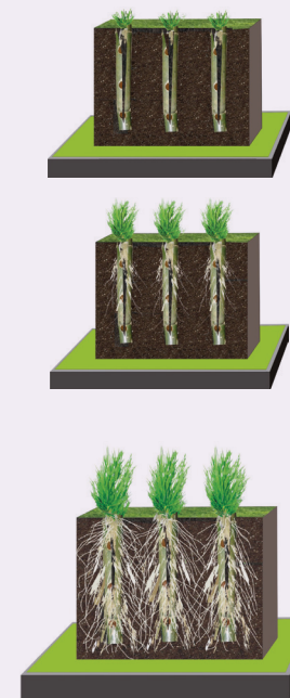
Vetiver grass implant in bamboo tubes.
