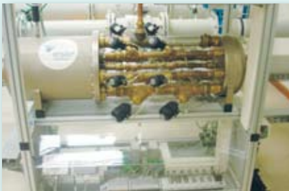
Compact reference sonic nozzle measuring unit
